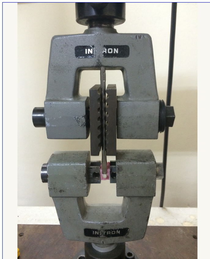
[Table/Fig-3]: Sample under universal testing machine
